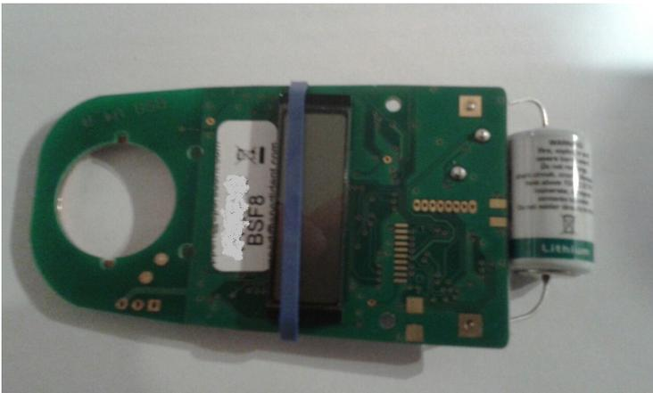
5. Now remove the old part – note the polarity of the item you are removing. You will probably need to use a soldering iron for this (unless replacing the screen).
