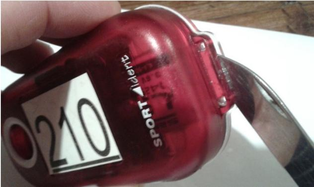
2. Carefully open up the case – if you don't want to replace the o-ring, then try to keep it in place by pressing on it with the blade. Otherwise pull it out and remove any silicon gel attached to it and the case.
