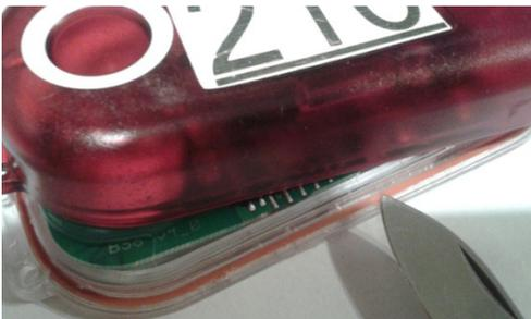
3. Unscrew the circuit board and put the 4 screws somewhere safe. Hopefully you now have the case in two parts (with or without the large o-ring), the motherboard and 4 screws.
